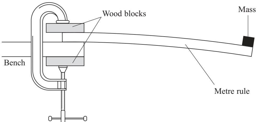
When pulled down a short distance and released, the cantilever will oscillate. The period of oscillation  $T$  will depend on the distance  $d$  of the mass from the clamped end, providing the mass on the end is kept constant.
